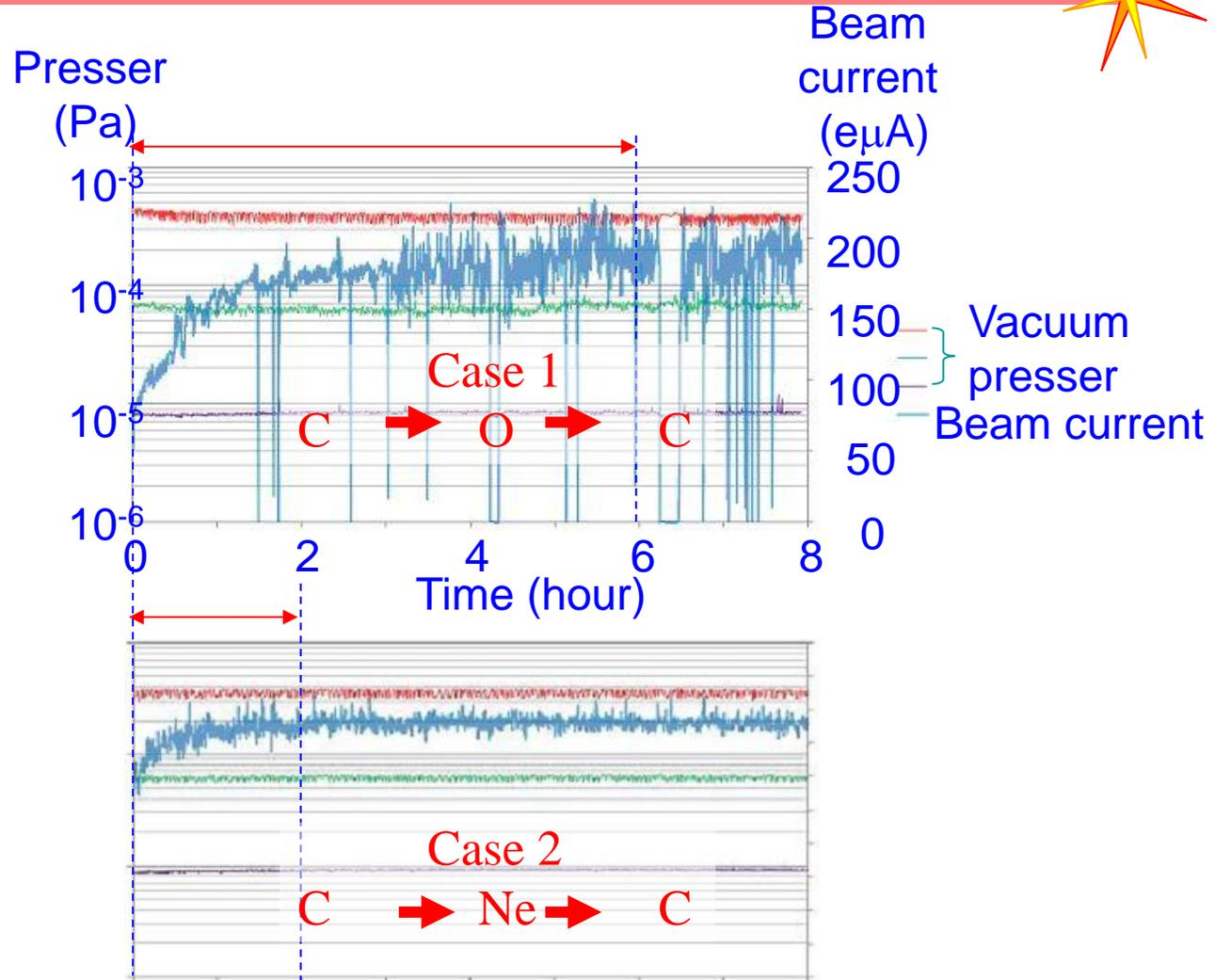
Carbon beam currents after the switching from oxygen and neon beam by Kei2.
