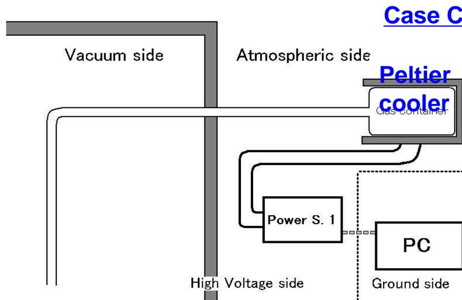
Block diagram of the cooling MIVOC system
