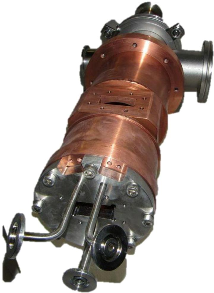
**Diagnostics box as a prechamber for hosting high sensitive/space resolved X-ray spectrometers**
