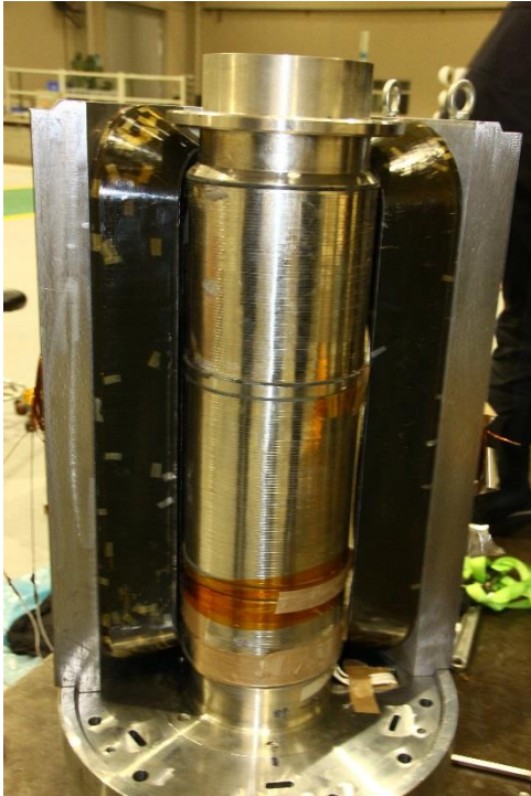
Sextupole Coils Pre-assembly
