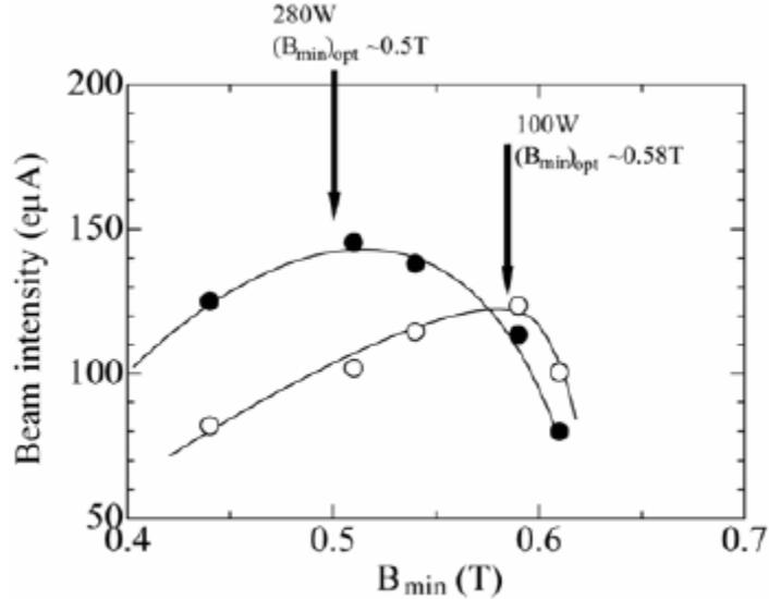
Fig.3 Beam intensity of  $Ar^{9+}$  as a function of  $B_{min}$  at the RF power of 100 and 280 W.
