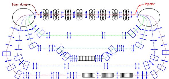
Figure 8: The third stage ERL with FEL undulators.
