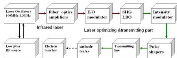
Figure 2: Schematic design of drive laser system.
