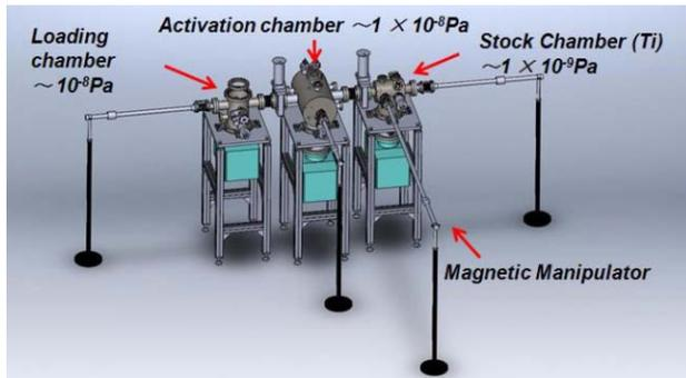
Figure 3: Structure of the photocathode preparation system.
