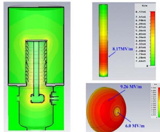
Figure 5: Simulation of E-field distribution by using CST.
