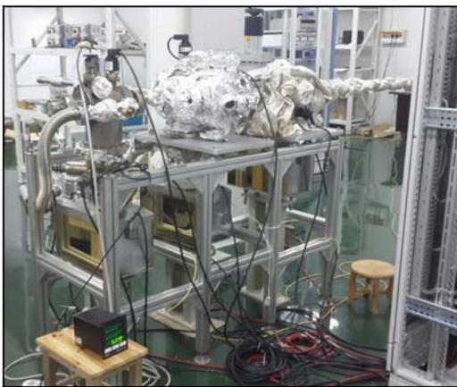
Figure 4: Baking and vacuum test of preparation system.
