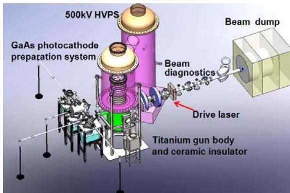
Figure 1: Overall design of the photocathode DC gun.
