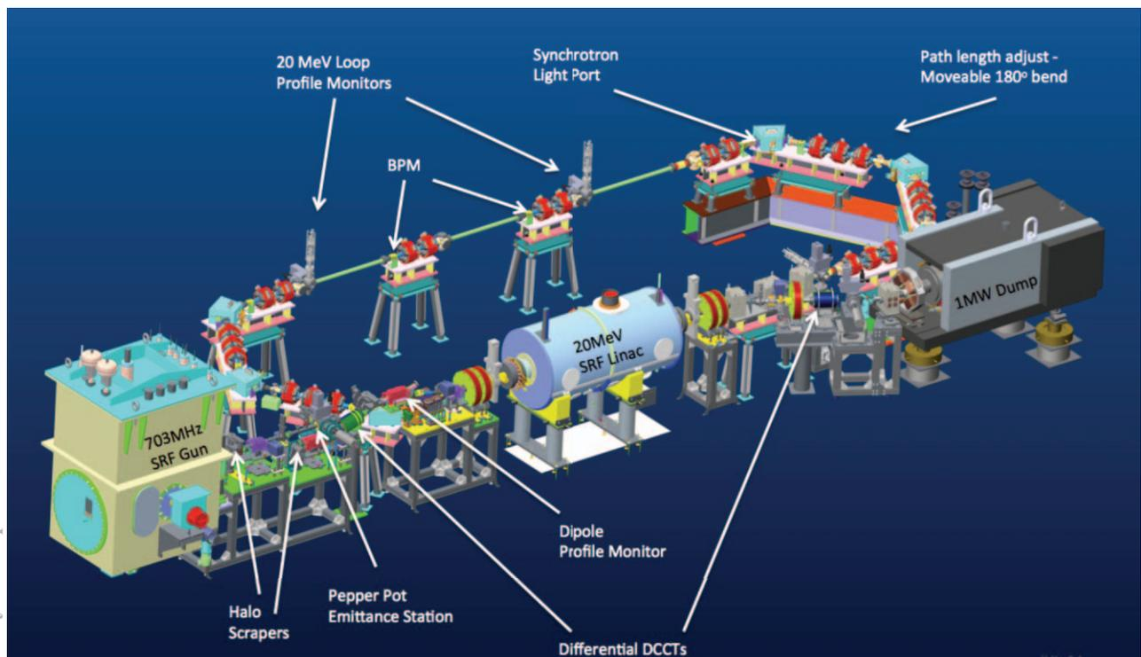
Figure 1: A 3D rendering of the ERL facility showing the SRF Gun, zig-zag injection transport, 5-cell SRF Linac, recovery loop, high power dump, and location details of some of the instrumentation detectors.
