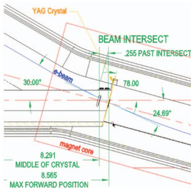
Figure 5: Injection Zig-Zag Dipole Profile monitor details, the electron beam trajectory in this view is right to left.
