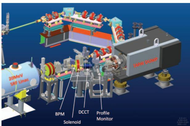
Figure 3: ERL 2MeV extraction line showing instrumentation locations.
