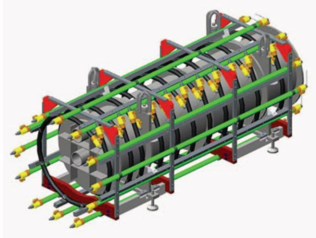
Figure 7: ERL Dump drawing showing the heliax cable type beam loss monitors shown in green and black.
