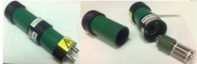
Figure 6: PMT based beam loss monitor detector, assembled at left, and disassembled.
