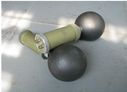
Figure 3: Ionization chamber.
