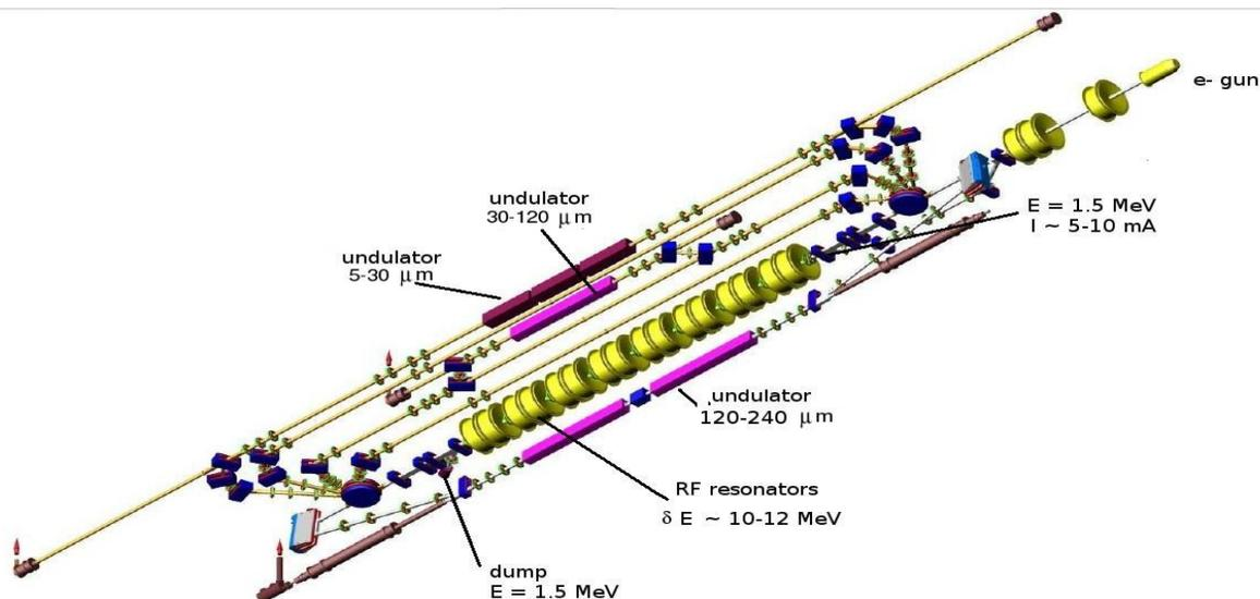
Figure 1: Novosibirsk ERL with the three FELs.
