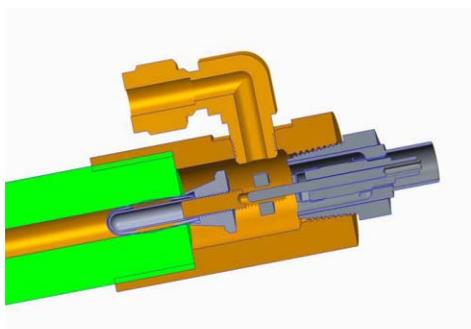
Figure 6: Rad-Hard BNC termination for 7/8 in. Heliac.
