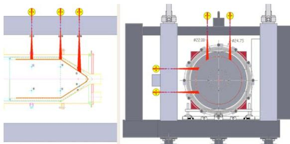
Figure 7: Pinhole radiation measurements: (left) top view, (right) axial view.
