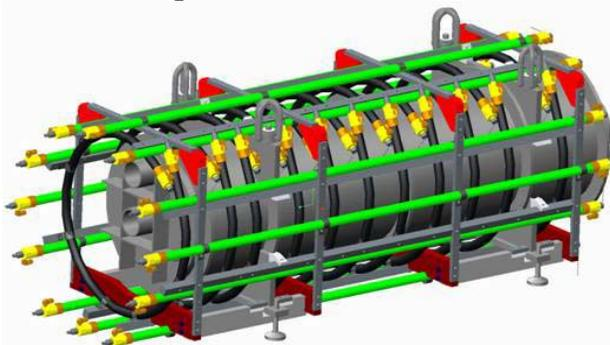
Figure 4: Beam Dump with Heliac BLM matrix.
