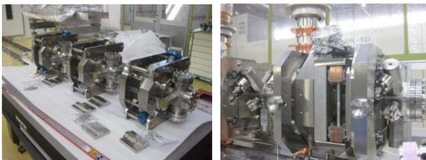
Fig. 5: Superconducting Cavities (left) and Frequency Tuner (right)
