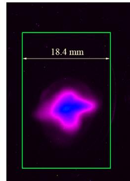
Figure 9: An example of the beam profile at a bunch charge of 7.7 pC, which was observed at a screen monitor “MS6” (after acceleration to about 5.6 MeV).
