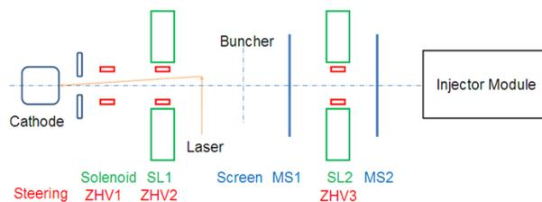
Figure 5: Setup of the emittance measurement of the beam from the photocathode DC gun.
