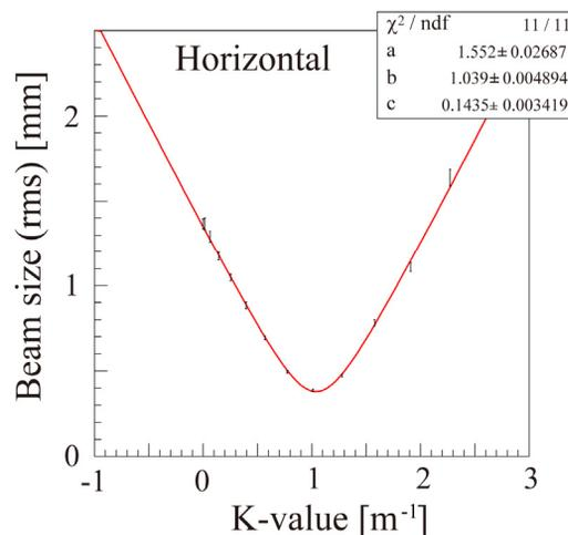
Figure 6: An example of the waist scan. Measured horizontal beam sizes at “MS3” are shown as a function of the focusing strength of the solenoid “SL2”.
