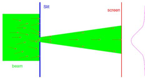
Figure 7: Schematic drawing of the slit-scan method.
