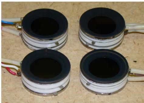
Figure 5: Photo of vacuum-sealed XHV - devises, which were used as a parallel-plate electron spectrometers.
