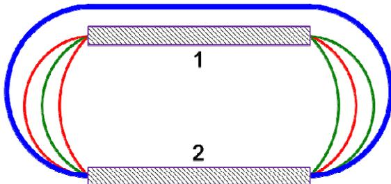
Figure 1: Scheme of ERL with two linacs.
