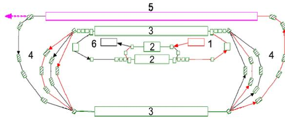
Figure 11. Recuperation groups of bunches: red – accelerating, blue – decelerating. 1-injector, 2 – two preinjection linacs, 3 – main linacs, 4 – bending arcs, 5 – undulator, 6 – beam dump.
