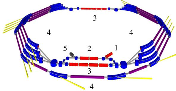
Figure 5: Scheme of MARS - ERL with two linacs: 1 – injector, 2 – preinjection linac, 3 – main linacs, 4 – bending arcs with undulators, 5 – dump.
