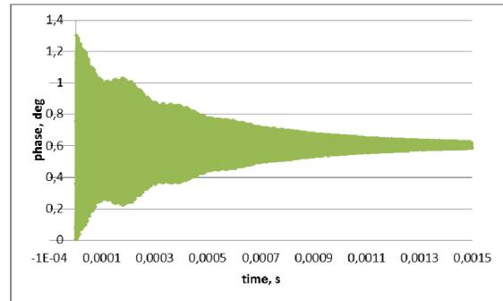
Figure 6: Example of the relaxation of the bunch's phase after the last deceleration to the equilibrium value.
