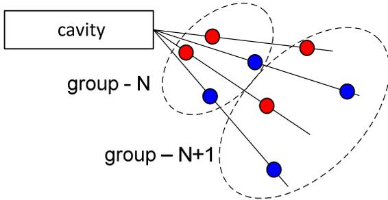
Figure 4. Recuperation groups of bunches: red – accelerating, blue - decelerating
