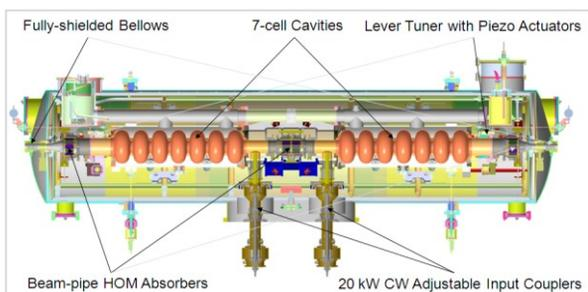
Figure 1: CW-ERL cryomodule under development.
