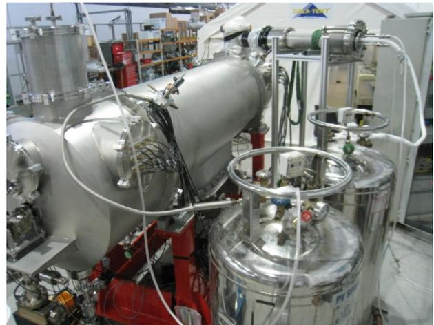
Figure 2: Fully assembled cryomodule undergoing Qualification tests.
