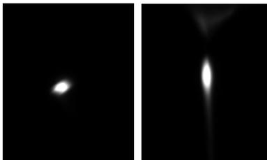
Figure 4: Original transverse beam (left), and longitudinal beam profile (right). RF and laser are synchronized. [5]
