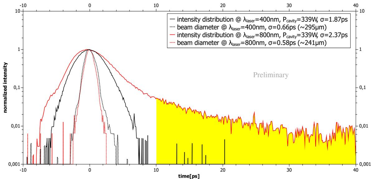
Figure 5: Longitudinal and transverse pulse profiles at  $\lambda_{\text{laser}} = 800 \text{ nm}$  (red) and  $\lambda_{\text{laser}} = 400 \text{ nm}$  (black) [5]. The yellow area shows the beam loss at the acceptance of an accelerator of  $\sigma_{\text{pulse}} = 10 \text{ ps}$ .
