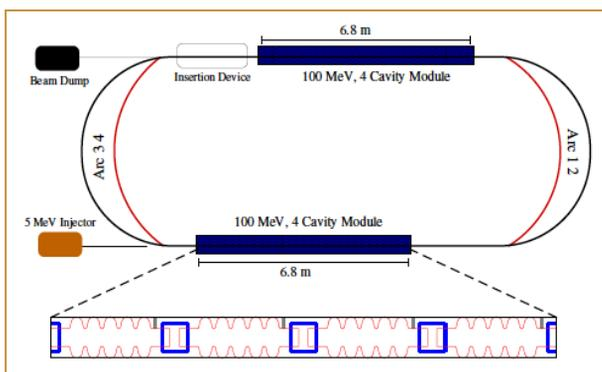
Figure 13: Schematic layout of an ERLTF at CERN [11].
