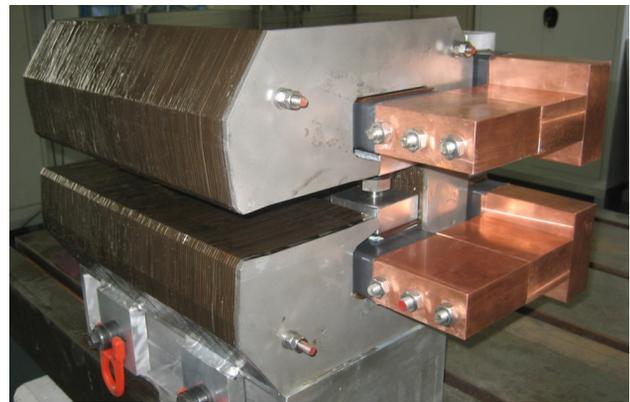
Figure 4: CERN prototype for a normal conducting LHeC dipole magnet.
