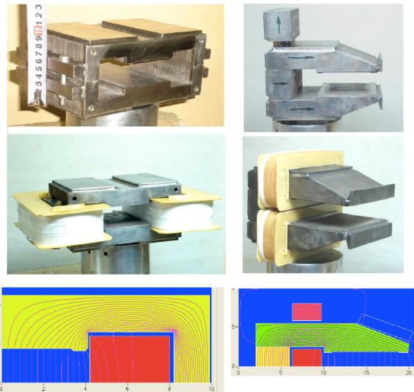
Figure 3: BINP prototype for a normal conducting LHeC dipole magnet.
