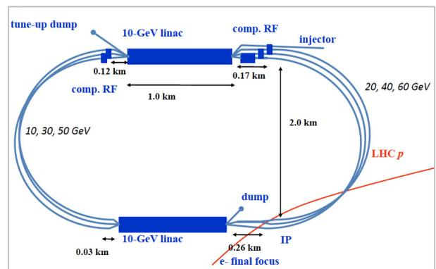
Figure 1: Schematic layout of the 60 GeV ERL option.
