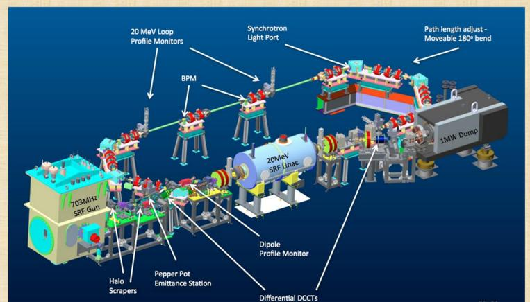
Above image is a 3D rendering of the ERL facility showing the SRF Gun, zig-zag injection transport, 5-cell SRF Linac, recovery loop, high power dump, and location details of some of the instrumentation systems.
