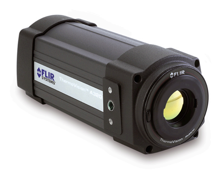
FLIR model A310 IR Camera, 320 x 240 px, Uncooled Microbolometer (7.5–13 μm spectrum)
