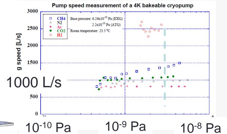
High pumping speed of bakable cryopump under extremely-high vacuum
