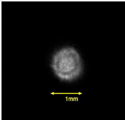
Laser profile at virtual cathode CCD camera.
