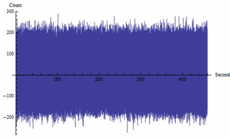
The amplitude stability is 2.8E-3 (peak-to-peak), or 2.3e-4 (rms).  The phase stability is 0.42° (peak-to-peak), or 0.035° (rms).
