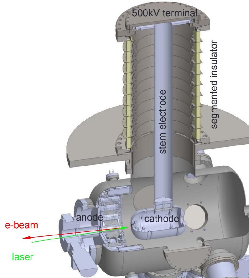
Operational voltage of photo-gun has been limited to 350kV since the first proposal of the 500kV photo-gun in 1991.
