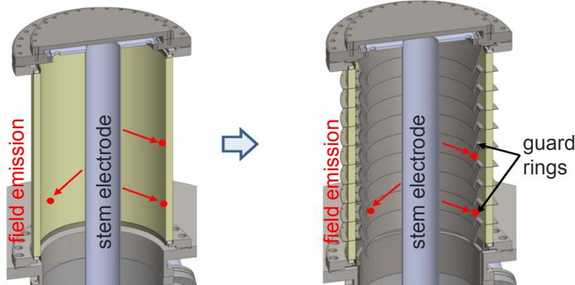
2: Discharge between the cathode and HV chamber (anode) which propels microparticles on the HV chamber surface to the cathode. The microparticles serve as a field emission site.
