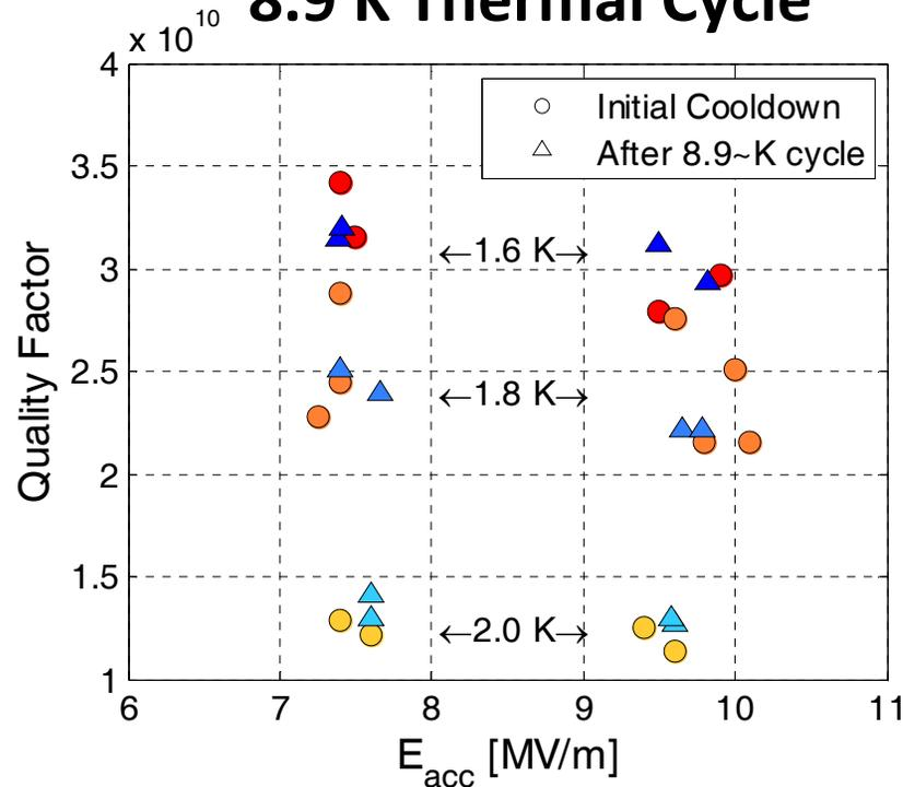
HTC-2 measurements did not find a statistically significant increase in Q for 8.9 K thermal cycle.
