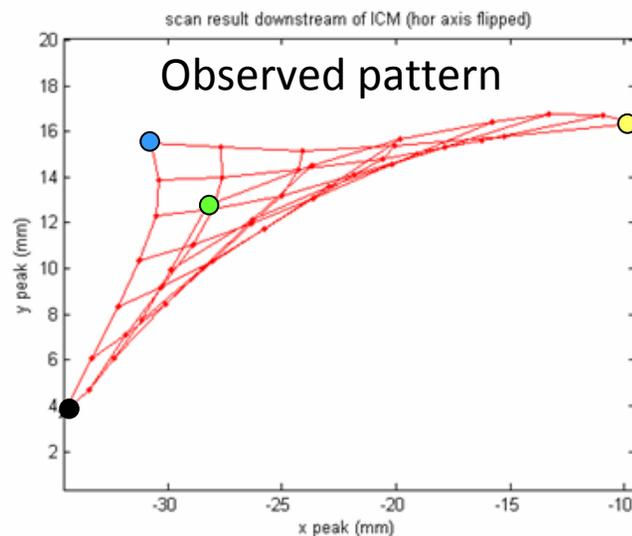
Rastering the beam in a square pattern in front of the cryomodule produce a distorted pattern after the cryomodule
