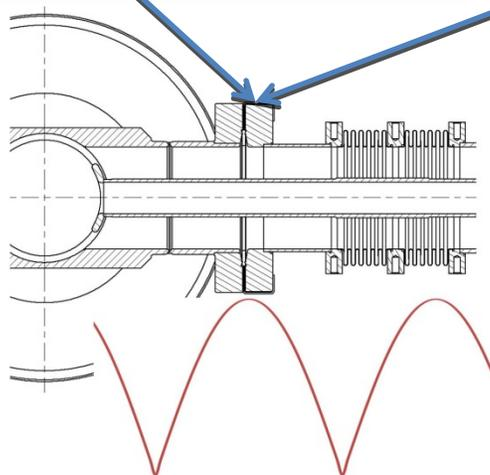
Standing wave max at the flange joint causes excessive heating. A new joint was designed for future couplers.
