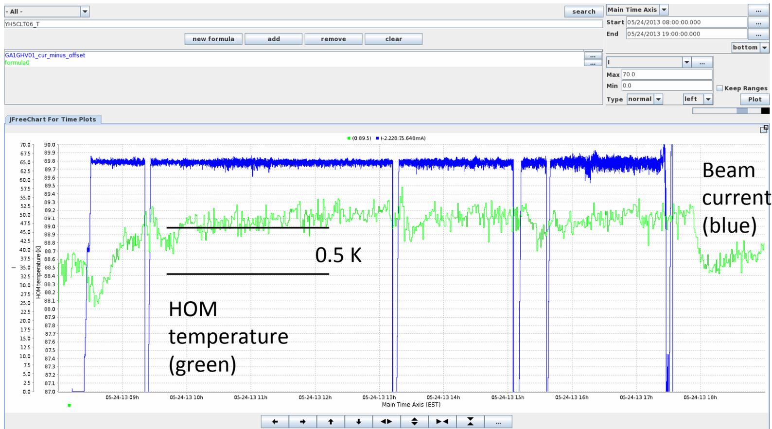
At most 0.5K temperature rise (65 mA, 4 MeV, 2-3 ps rms bunch length),
