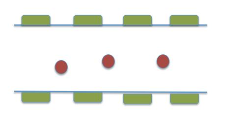
$$\begin{split} v_i &= \frac{U_{up\,i} + U_{up\,i+1} - U_{down\,i} - U_{down\,i+1}}{U_{up\,i} + U_{up\,i+1} + U_{down\,i} + U_{down\,i+1}} \\ h_i &= \frac{U_{up\,i} - U_{up\,i+1} + U_{down\,i} - U_{down\,i+1}}{U_{up\,i} + U_{up\,i+1} + U_{down\,i} + U_{down\,i+1}} \end{split}$$
