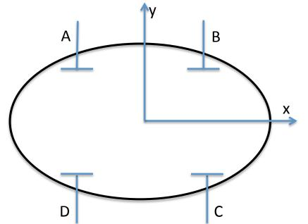
$$x_{diff} = \frac{k_x}{\tan(\omega \Delta t_{12}/2)} [(\varphi_B - \varphi_D) - (\varphi_A - \varphi_C)]$$
