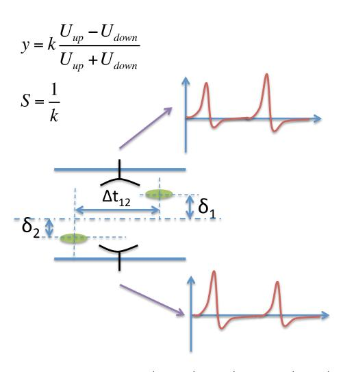
Bunches, separated by a flyby time  $\Delta t_{12}$ , have different positions then each PUE sees different longitudinal "center of gravity" and there is a phase shift between two signals. For a processing unit, utilizing signal processing at frequency ω, and small displacements of the first and the second bunches  $\delta_1$  and  $\delta_2$  (S $\delta_1$ ,S $\delta_2$   $\ll$  1, where S=1/k is a sensitivity coefficient) we can write the linearized equations:
