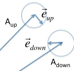
When the measurement error is not correlated with the signal the probable error will draw a circle around the end of the vector and r.m.s. phase error will be equal to the signal to noise ratio of the amplitude measurement  $\sigma_{\varphi} = \frac{\sigma_A}{\Delta}$
