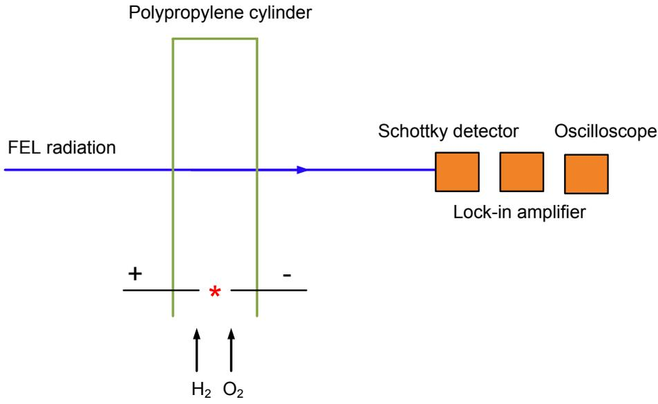
Combustion H<sub>2</sub>- O<sub>2</sub> mixer in Ø40×200 mm polypropylene cylinder
