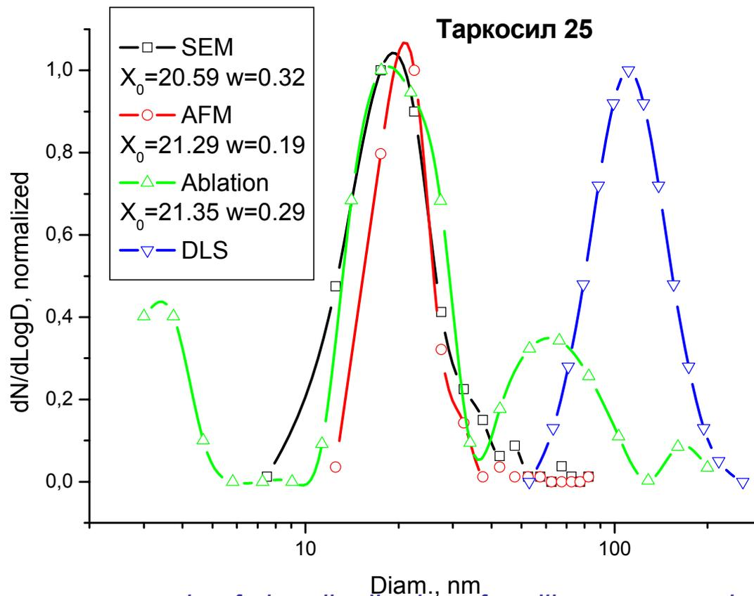
*The slide presents an example of size distributions for silica nanopowder produced in BINP. Soft ablation demonstrates the excellent agreement for main fraction of particles and aggregates and confidently registers a difficult fraction of 3-5 nm. It should be noted that the method of soft ablation do not require complex and time-consuming steps of sample preparation and analysis. Single measurement takes 4 minutes.*
