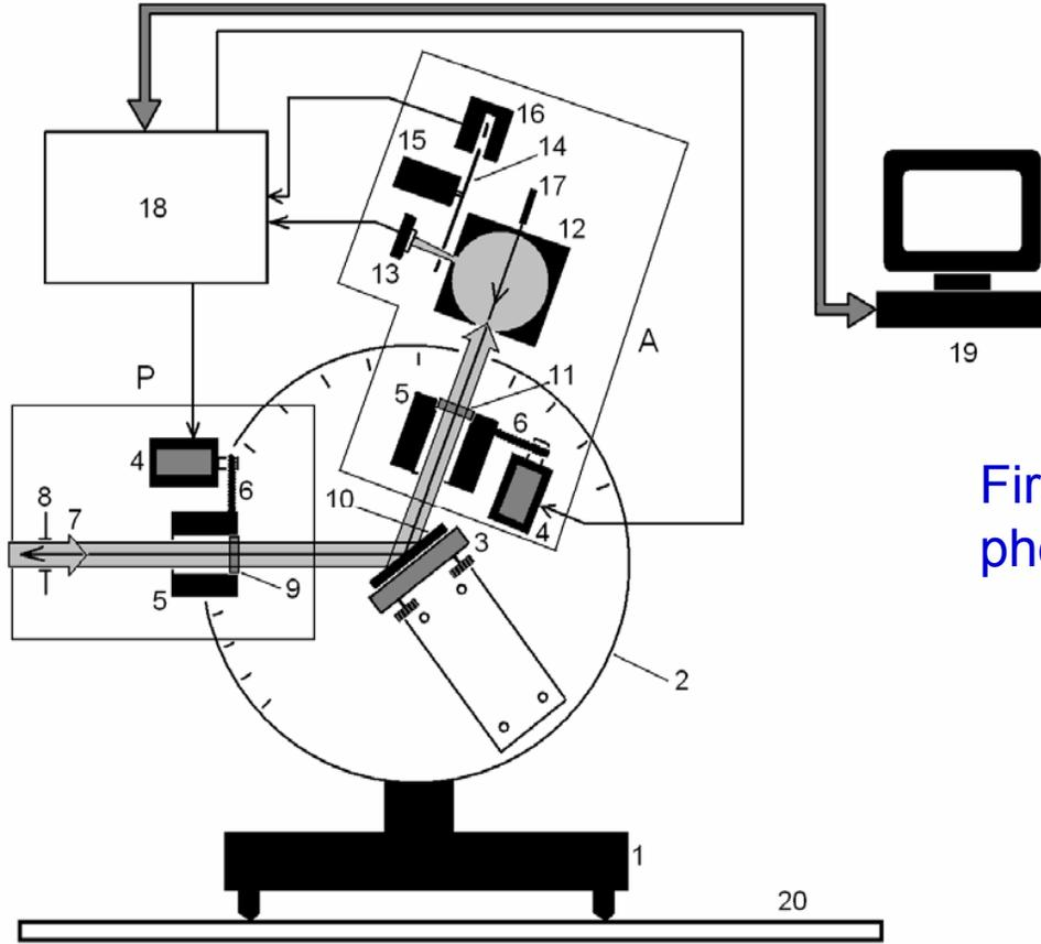
Ellipsometry measures the complex reflectance ratio,  $\rho$ , of a system, which may be parametrized by the amplitude component  $\Psi$  and the phase difference  $\Delta$ .
