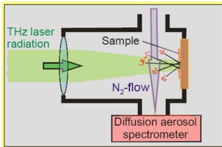
Demonstration of ultra-soft ablation of DNA samples without defragmentation: when the power density of THz radiation is optimal, particle size spectra contain only the peaks corresponding to the initial particles.
