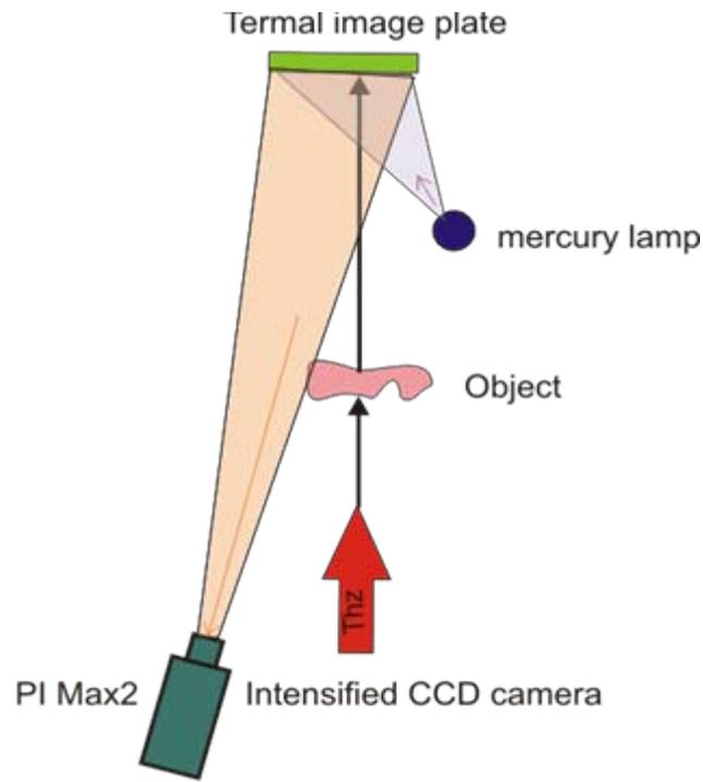
Experiments have been performed using classical scheme in line (Gabor) holography. Holograms were recorded using temperature sensitive phosphor image plate with a CCD camera and then numerically reconstructed by calculation the Fresnel-Kirchhoff integral in the real image plane.
