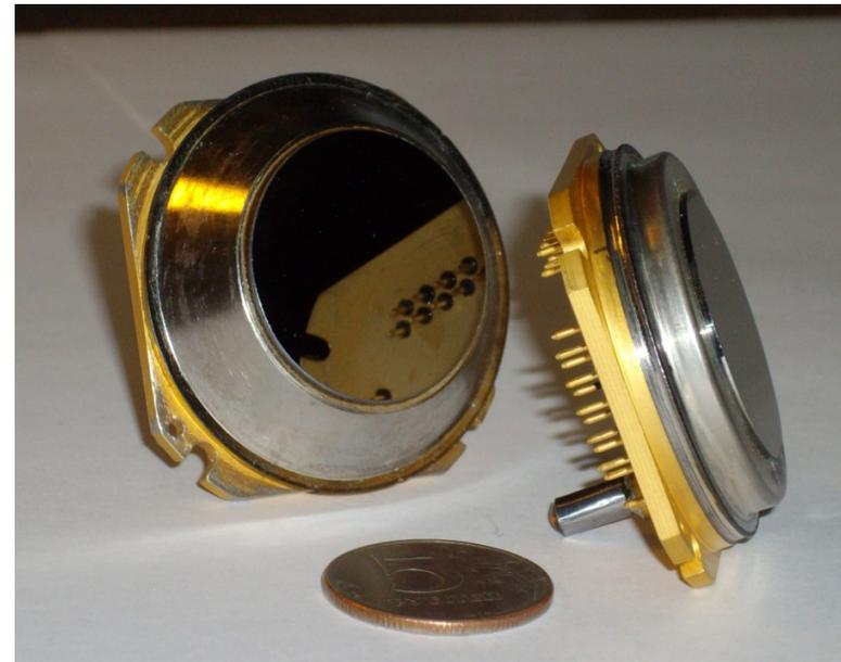
Two samples of microbolometer FPA
