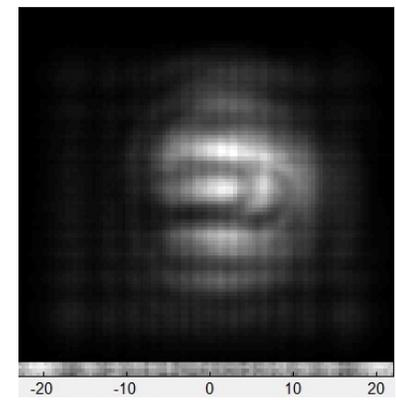
Amplitude distribution in the reconstructed real image plane
