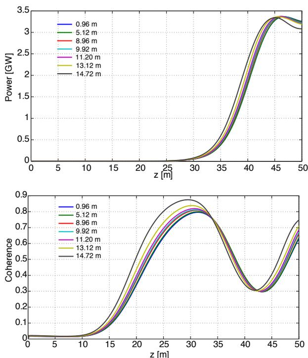
Figure 4: FEL power and coherence of a 1 nm X-ray FEL for various cell lengths of the FODO lattice (upper and lower plot, respectively).
