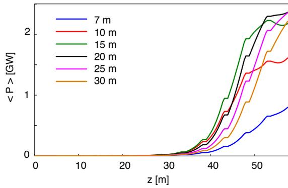
Figure 2: FEL performance of the SwissFEL 1 Å X-ray FEL for various focussing strengths of the FODO lattice, expressed by its average beta function.
