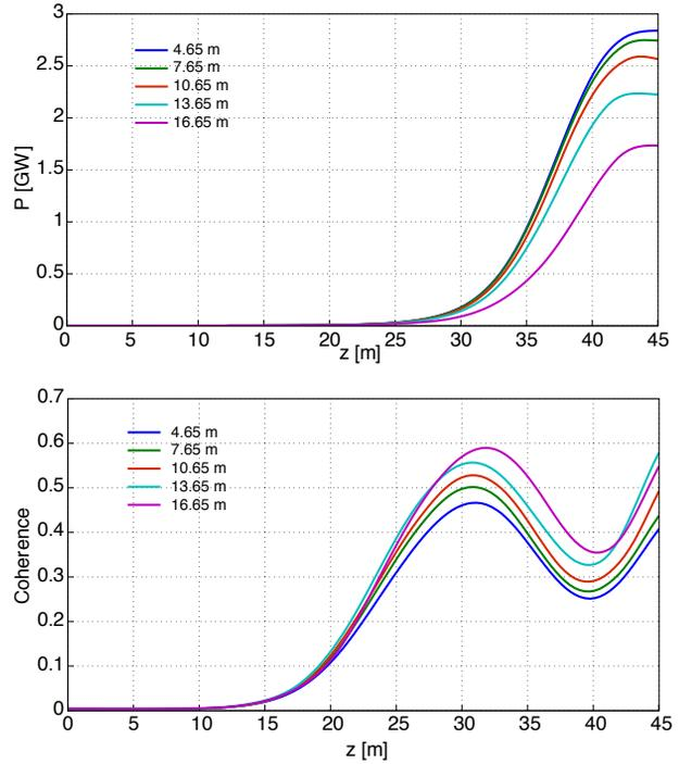
Figure 3: FEL power and coherence of an 1 Å X-ray FEL for various cell lengths of the FODO lattice (upper and lower plot, respectively).
