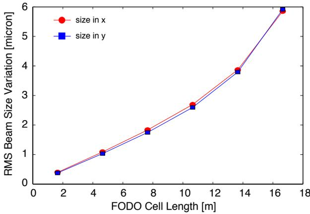
Figure 1: Beam size variation for different cell lengths of the FODO lattice, based on the SwissFEL hard X-ray FEL parameters.
