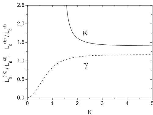
Figure 1: Ratio of gain lengths of the retuned fundamental and the third harmonic for lasing at the same wavelength versus rms undulator parameter  $K$ . The fundamental wavelength is reduced by means of reducing the undulator parameter  $K$  (solid) or increasing beam energy (dash).
