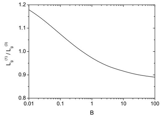
Figure 2: Ratio of gain lengths for lasing at the fundamental wavelength and at the third harmonic versus diffraction parameter of the fundamental wavelength for large values of the undulator parameter  $K$ .
