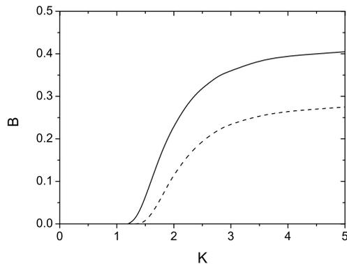
Figure 3: Diffraction parameter of the fundamental wavelength, for which the third (solid) and the fifth (dash) harmonics have the same gain length as the fundamental, versus the rms undulator parameter  $K$ . Below these curves harmonics have shorter gain lengths than the fundamental frequency.
