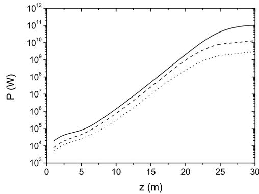
Figure 4: An example for the European XFEL. Averaged peak power for the fundamental harmonic (solid), the third harmonic (dash), and the fifth harmonic (dot) versus undulator length for SASE3 operating at 4.5 nm. Parameters are in the text. Simulations were performed with the code FAST.
