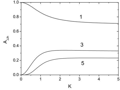
Figure 1: Coupling factors for the 1st, 3rd, and 5th harmonics (denoted by 1, 3, and 5, correspondingly) versus rms undulator parameter.
