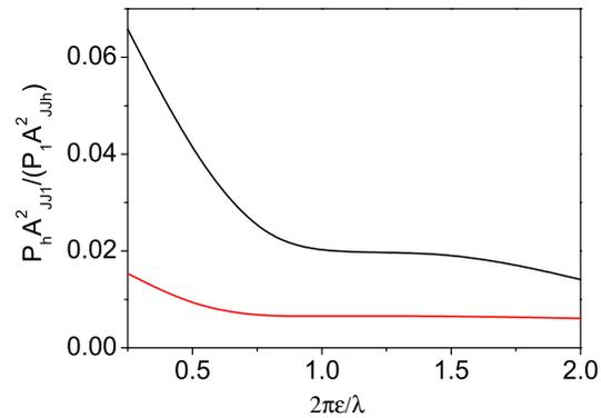
Figure 3: Optimized XFEL. Ratio of powers in the 3rd (black line) and the 5th harmonic (red line) to the power of the fundamental harmonic versus parameter  $\epsilon = 2\pi\epsilon/\lambda$ . SASE FEL operates at the saturation point.
