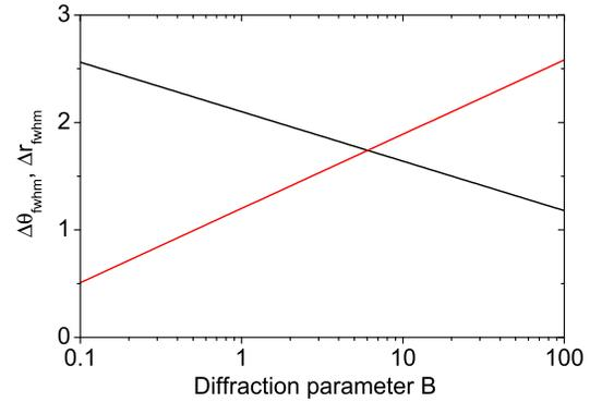
Figure 2: Normalized FWHM size (black curve) and angular divergence (red curve) of SASE FEL radiation versus diffraction parameter. SASE FEL operates at the saturation point.
