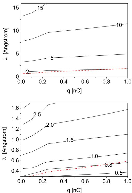
Figure 6: FWHM angular divergence of the radiation for SASE1 (top) and SASE3 (bottom) FELs operating in the saturation versus bunch charge and operating wavelength. Electron energy is 17.5 GeV. Numbers on contour lines denote units of  $\mu\text{rad}$ . Red dashed curve shows minimum of the radiation wavelength at the undulator length of 165 m. Parameters of the electron beam are presented in Table 1. Focusing beta function is optimized for minimum gain length.
