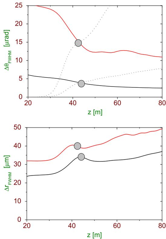
Figure 1: Radiation spot size (bottom) and angular divergence (top) of the radiation versus undulator length for SASE1 (SASE3). Black and red curves refer to the case of SASE1 and SASE3, respectively. Parameters of SASE1 (SASE3) are: electron energy is 14 GeV (17.5 GeV), bunch charge is 100 pC, wavelength is 0.25 nm (1.6 nm). Dotted lines show radiation pulse energy. Circles denote saturation point.
