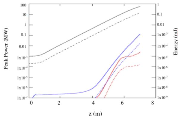
Figure 4: Nominal case. No phase shifts, no  $K$  variation. Black: Fundamental, Blue: 3<sup>rd</sup> Harmonic, Red: 5<sup>th</sup> Harmonic. Solid: Peak Power, Dashed: Energy.
