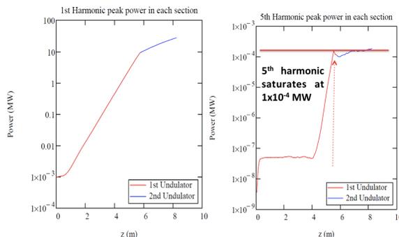
Figure 7: Saturation is a magnitude of one order less than without phase shift
