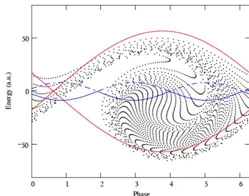
Figure 3: Longitudinal phase space plot of the FEL microbunching including the computed separatrices for the fundamental (red) and 3<sup>rd</sup> harmonic (blue).
