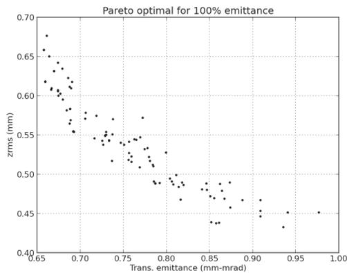
Figure 2: Pareto front for the 300 pC nominal charge. Quantities plotted at the exit of the injector (15 m from the cathode, energy > 90 MeV)
