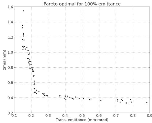
Figure 5: Pareto front for the low charge (30 pC) operating mode
