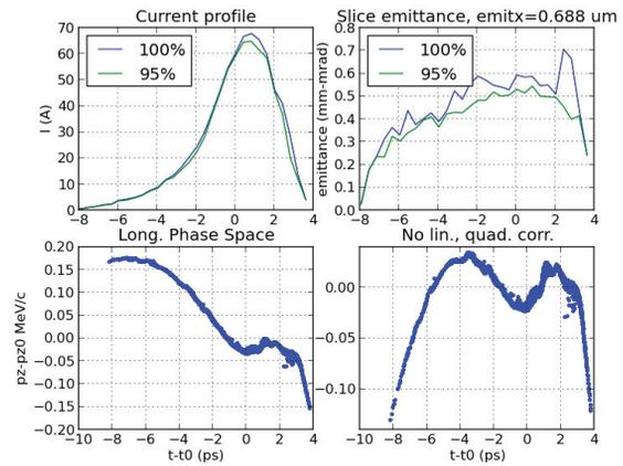
Figure 3: High compression solution for 300 pC bunch charge
