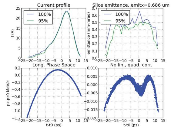
Figure 4: Low compression solution for 300 pC bunch charge. Compare with Fig. 3
