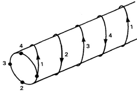
Figure 1: Quadrupole wiggler configuration
