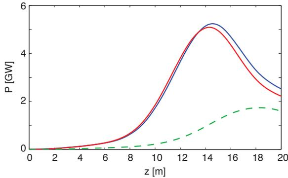
Figure 5: Time-dependent simulation of the second stage in a HGHG configuration, operating at the 50th harmonics (red curve). For comparison the slice-averaged results are shown for nominal current (blue curve) and reduced current (green dashed line).
