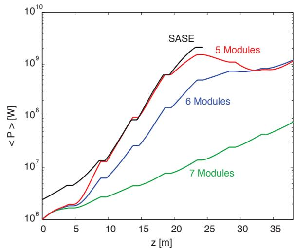
Figure 2: FEL power along the second stage for various lengths of the first stage. The SASE performance has been shifted in position for better comparison.
