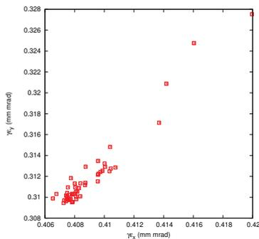
Figure 5: Vertical and horizontal normalized emittance for case with all quadrupoles and sextupoles are random misaligned (Isochronous lattice). For the displacements we used a gaussian distribution with RMS width of  $50 \mu m$ . This represent the worse lattice in term of sensitivity to magnets alignment.
