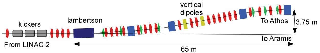
Figure 1: Schematic layout of Athos Switchyard. (blue) horizontal dipoles and lambertson, (yellow) vertical dipoles, (red) quadrupoles, (green) sextupoles.
