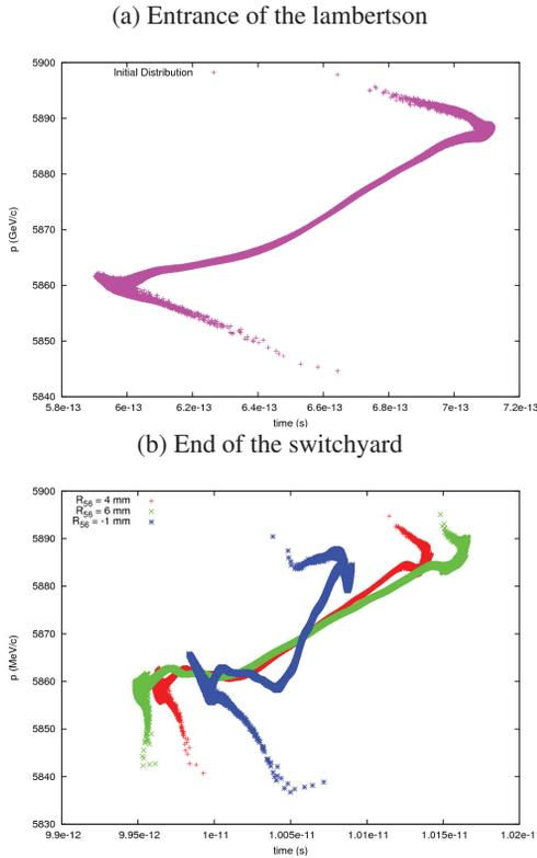
Figure 4: Initial (a) and final longitudinal (b) phase space for different values of  $R_{56}$ . The CSR effects are visible in all cases.
