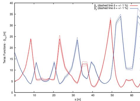
Figure 2: Lattice functions for the case with  $R_{56} = 4$  mm. The dashed line are the twiss functions for particles with energy difference of  $\delta_E = \pm 1.0\%$ .
