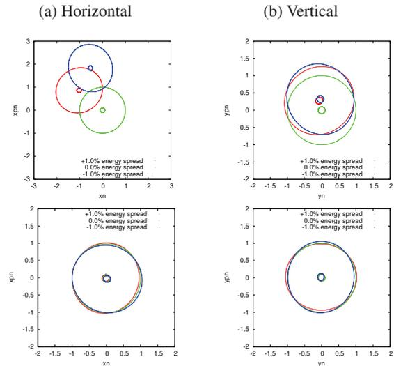
Figure 3: Non linear effects present on the lattice. The plots show the horizontal and vertical phase space for 0.1 and  $1\sigma$  ellipses and for on energy particles (green dots) and  $\delta_E = \pm 1.0\%$  (red and blue dots), (top) sextupoles off and (bottom) sextupoles on.
