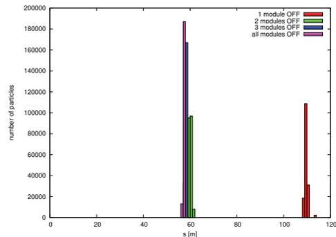
Figure 6: Loss map for the switchyard as we turn off, one by one, the last four modules in Linac 2. In the plot the coordinate system begins at the entrance of Linac 2, the switchyard starts are  $s = 55$  m.
