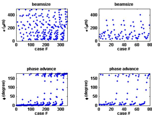
Figure 4: Simulation result with current quadrupole setup. Beamsize (Top) and phase advance (Bottom) at the position of the screen with different quadrupole strength. The quadrupole strength values are  $-3/m^2$  to  $3/m^2$  with  $1/m^2$  step from left to right. Beamsize after eliminating
