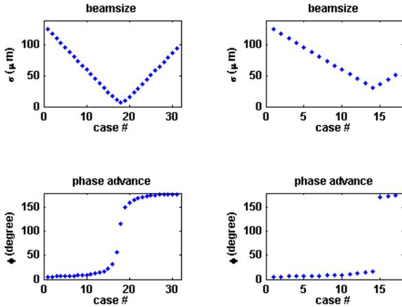
Figure 3: Simulation result with single quadrupole. Beamsize (top left) and phase advance (bottom left) at the position of the screen with different quadrupole strength. quadrupole strength values are  $-4/m^2$  to  $4/m^2$  with  $0.25/m^2$  step from left to right. Beamsize after eliminating overlapped cases (top right) and its phase advance (bottom right).
