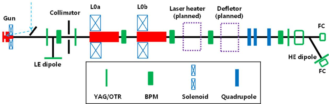
Figure 1: Schematic layout for the ITF beamline.
