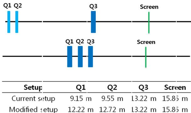
Figure 2: Current quadrupole setup (Top) and modified.
