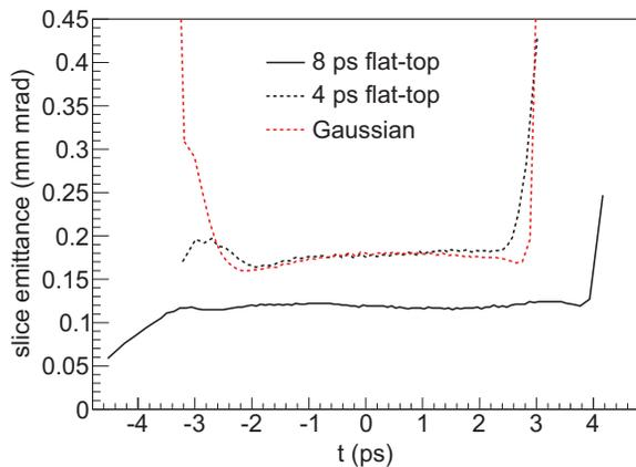
Figure 7: Normalized transverse slice emittance of 200 pC bunches at the injector end.
