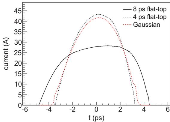
Figure 6: Current profiles of 200 pC bunches at the injector end for the three longitudinal profile options of cathode laser pulses.
