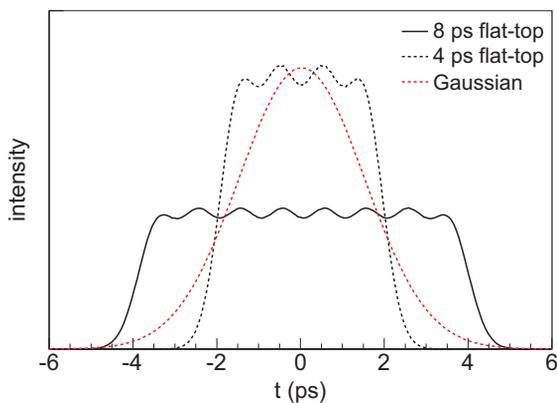
Figure 3: Longitudinal laser pulse profiles used for injector beam dynamics simulations. 8 ps flat-top is achieved by stacking 8 Gaussian pulses and 4 ps is by 4 pulses. As first phase operation, a simple 1.5 ps rms Gaussian pulse may be used.
