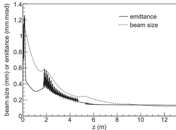
Figure 5: Beam size and normalized transverse projected emittance for the 200 pC nominal case.
