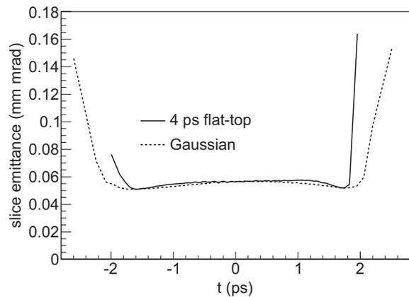
Figure 9: Normalized transverse slice emittance of 20 pC bunches at the injector end.
