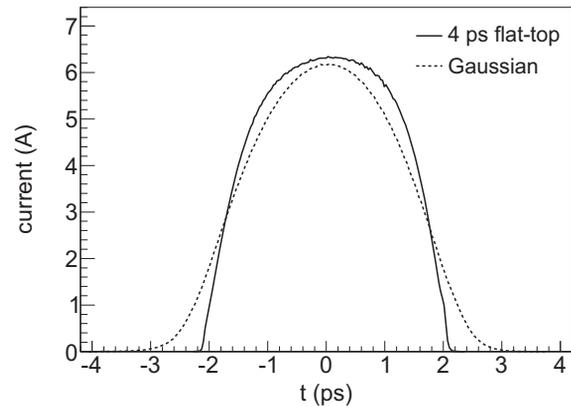
Figure 8: Current profiles of 20 pC bunches at the injector end.
