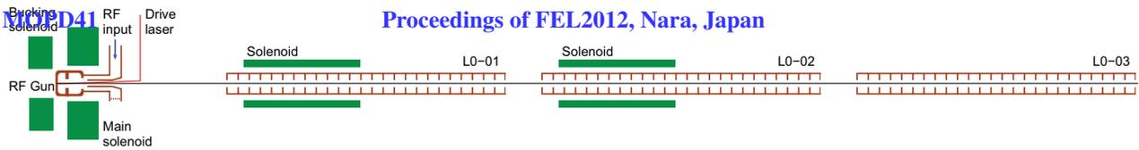
Figure 2: Layout of the low emittance injector consisting of an RF photocathode gun, focusing solenoids, and three accelerating sections.
