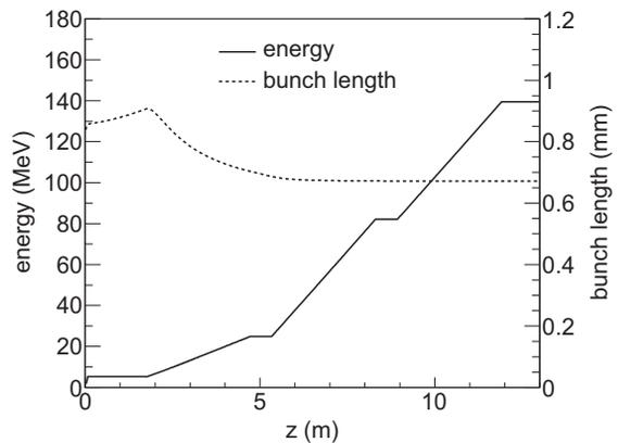
Figure 4: Beam energy and bunch length evolution for the 200 pC nominal case using a 8 ps flat-top laser pulse.
