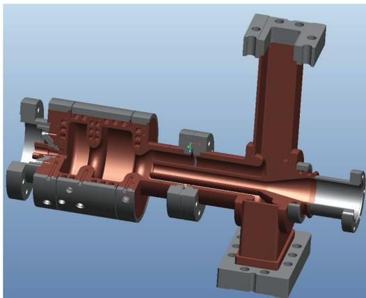
Figure 6: Alternative photocathode RF-gun.
