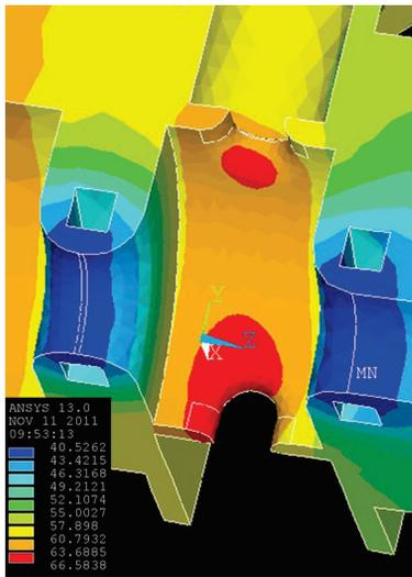
Figure 5: (Color online) Temperature distribution of the RF-gun. The maximum temperature gradient is about 26 °C
