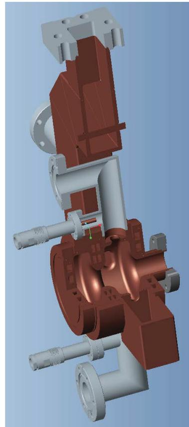
Figure 1: Three dimensional model of new photocathode RF-gun.
