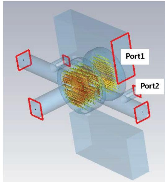
Figure 4: The simulation model of the new RF-gun and the electric field profile in the gun.
