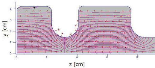
Figure 2: Field distribution in the RF-gun as calculated by using SUPERFISH.
