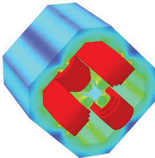
Figure 2: Magnetic distribution of quad (Q22-20).
