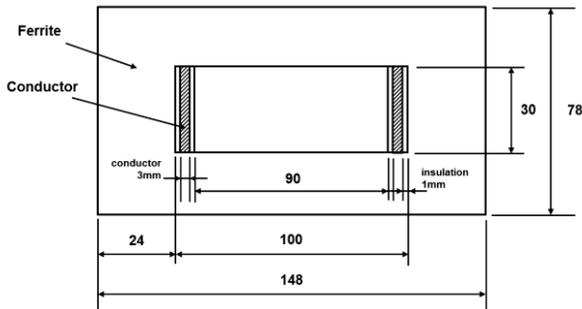
Figure 4: Core and coil size of kicker magnet.
