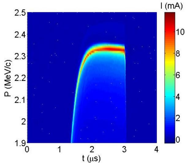
Figure 3: Measured 2D momentum spectrum. The leading edge of RF pulse corresponds to  $t = 1 \mu$ s.
