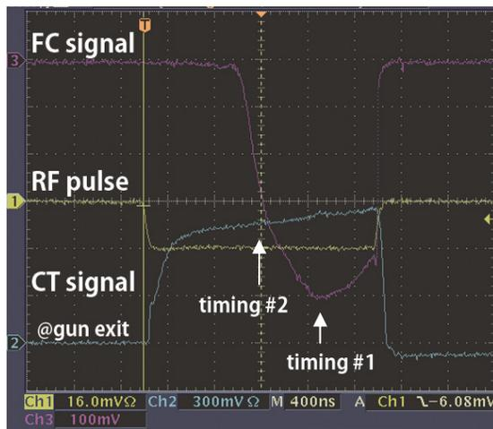
Figure 5: Observed beam signal. Ch.1: input RF pulse for cathode cell, Ch.2: CT signal and Ch.3: FC signal, respectively. Two different timings were assigned to measure the beam stability.
