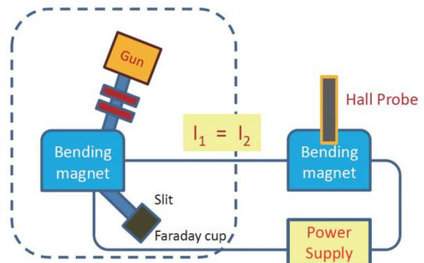
Figure 1: Measurement setup.
