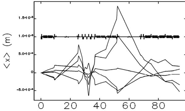
Figure 5: SXFEL beam trajectory before correction: 5 particles, 30 BPMs.
