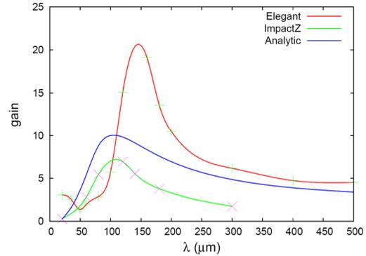
Figure 7 (color):  $\mu\text{BI}$  gain in SXFEL computed by different methods: Elegant (red), ImpactZ (green) and Analytic (blue).
