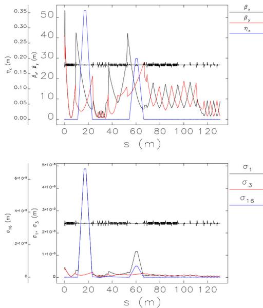
Figure 3 (color): upper: betatron functions:  $\beta_x$  (black);  $\beta_y$  (red) and  $\eta_x$  (blue) along the LINAC; Lower: beam envelope functions:  $\sigma_1$  (black),  $\sigma_3$  (red),  $\sigma_{16}$  (blue).
