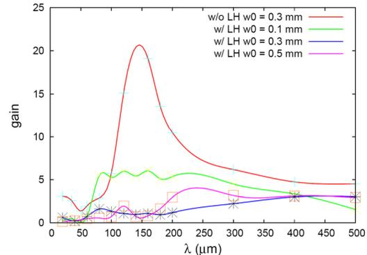
Figure 8 (color):  $\mu\text{BI}$  gain in SXFEL computed by Elegant with various laser waist sizes: without laser heater & waist = 0.3 mm (red), with laser heater & waist = 0.1 mm (green), with laser heater & waist = 0.3 mm (blue), with laser heater & waist = 0.5 mm.
