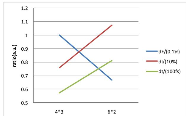
Figure 4 (color): comparison of jitters at different compression rate assignments (BC1\*BC2).
