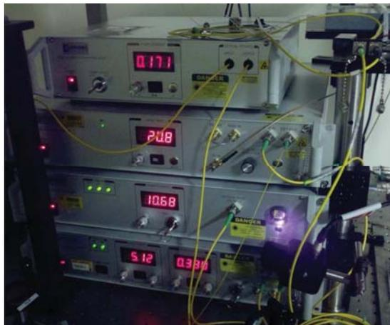
Figure 2: Picture of the fiber based seed laser setup the bottom to top it's seed oscillator, power amplifier, pulse picker and preamplifier respectively.
