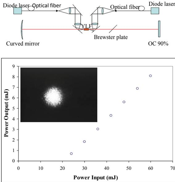
Figure 5: Top sketch is the end pumped 1053 nm Nd:YLF laser resonator layout. Bottom shows measured output energy vs. the pump energy. The inset shows the spatial profile from our TEM<sub>00</sub> mode captured using a CCD camera
