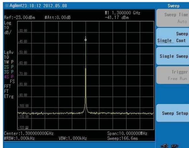
Figure 3: RF spectrum of the seed laser locked at at 1.3GHz.
