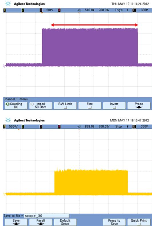
Figure 6: Scope image of the multi-pass input (top) and multipass output (bottom). The pulse energy is 1 nJ at the input and above 2μJ after the multi-pass cavity. The red arrow indicates a length of 1ms.
