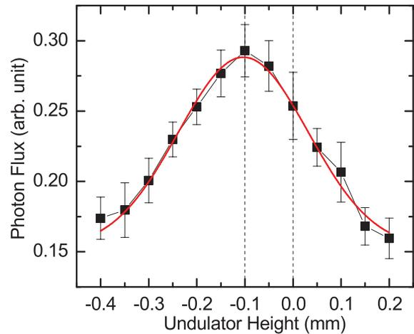
Figure 5: Photon flux of spontaneous radiation from the 1st segment measured at 10 keV as a function of the undulator height (black square). The result of Gaussian fitting is also indicated (red line).
