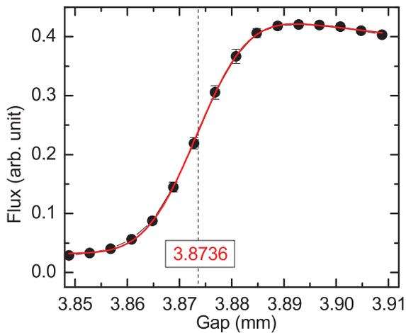
Figure 4: Photon flux of spontaneous radiation from the 1st segment measured at 10 keV as a function of the gap (black circle). The results of fitting is also indicated (red line).
