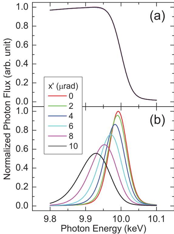
Figure 3: Example of calculated spectra of spontaneous radiation emitted from the 1st segment in two different slit aperture sizes: (a) 10 mm and (b) 0.5 mm.
