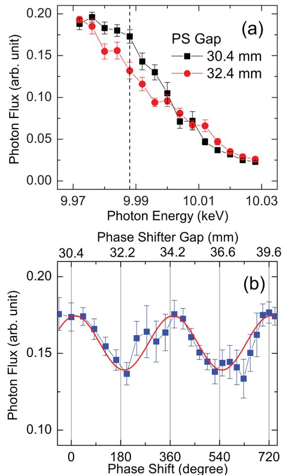
Figure 6: Phase matching example. (a) Spectra of spontaneous undulator radiations for two different gap values of the phase shifter installed in between, when the 1st and 2nd segments have the identical K values of 2.1. (b) Photon flux at 9.988 keV measured as a function of the relative phase shift (blue square). The phase shifter gap corresponding to the phase shift of  $n\pi$  is indicated in the top scale. The sinusoidal fitting of the measured result is also shown (red line).
