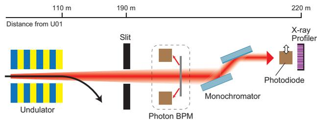
Figure 1: Schematic illustration of the photon diagnostics system in SACLA.
