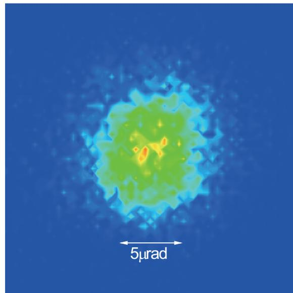
Figure 2: Example of a single-shot image of monochromatized spontaneous radiation from the 1st undulator segment, taken by the CCD detector.
