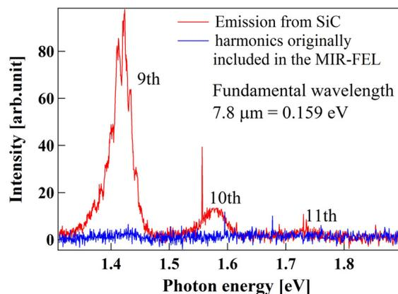
Fig 5: Emission from SiC and harmonics originally included in the MIR-FEL.
