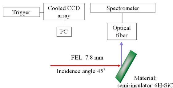
Figure 3: Measurement setup of HHG from SiC.
