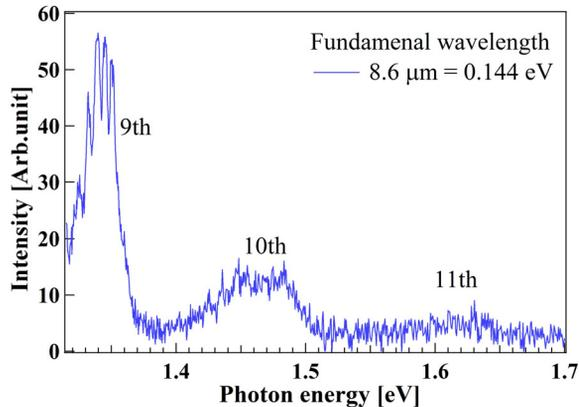
Figure 6: Spectra of the emissions from SiC irradiated by MIR-FEL whose wavelength was 8.6  $\mu\text{m}$ .
