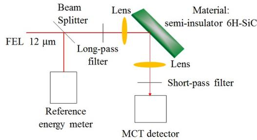
Figure 2: Measurement setup for verification of the SHG.
