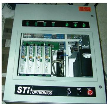
Figure 3: IR and UV wiggler control rack.
