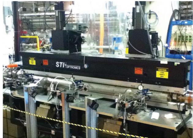
Figure 1: UV wiggler installed at JLAB.
