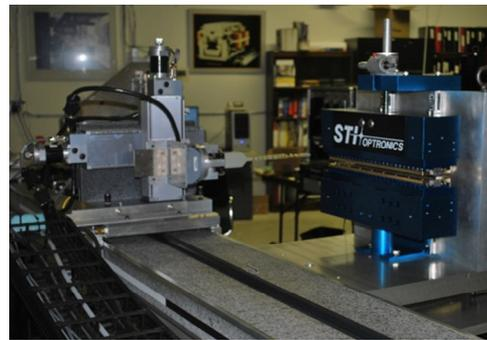
Figure 1: 55 mm (left, on NLCTA) and 33 mm (right, being scanned) period undulators.
