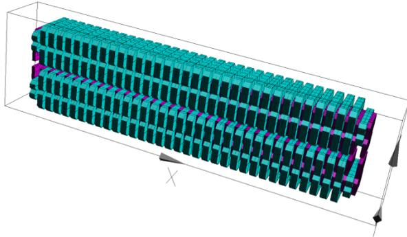
Figure 6: Shortened RADIA model of the undulator.
