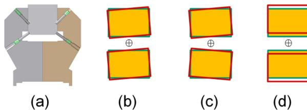
Figure 8: Tuning scheme. (a) shows the tuning studs and locking studs for the pole. (b) shows the correction scheme for skew dipole (c) shows the correction scheme for normal quadrupole (d) shows the correction scheme for dipole or orbit.
