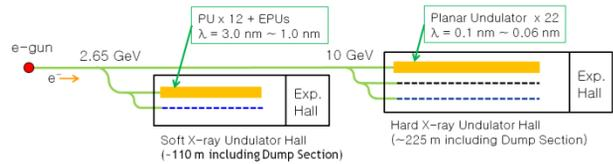
Figure 1: Schematic layout of the PAL-XFEL and undulator line.
