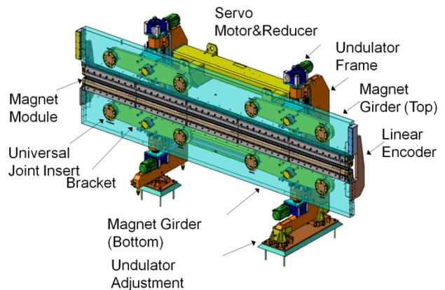
Figure 2: Schematic structure of PAL-XFEL undulator system.
