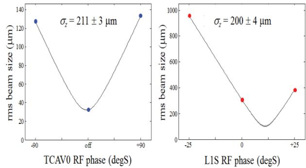
Figure 7: Measured rms beam sizes in *LCLS* injector at 20 pC vs. RF phase (transverse cavity phase at left, and pre-BC1 accelerating phase, L1S, at right). The two independent bunch length measurements agree to within 5% here.
