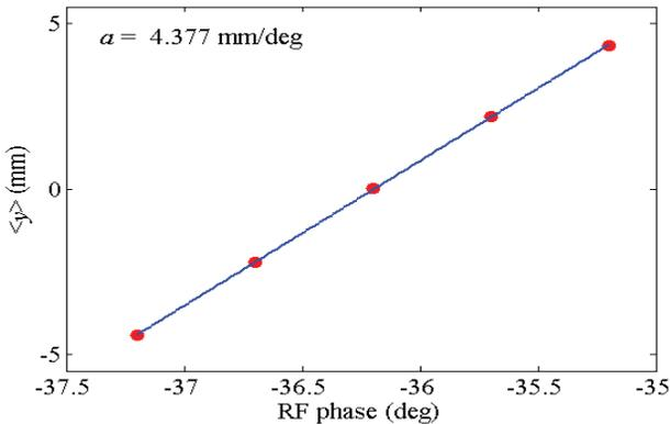
Figure 1: Simulated calibration curve as described in Eq. (5) with  $a = 4.377$  mm/deg (or 250.8 mm/rad).
