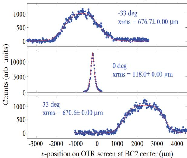
Figure 10: Measured temporal profiles for an L2 RF phase of  $-33^\circ$  (top), zero (middle), and  $+33^\circ$  (bottom) at 40 pC in the BC2 chicane (same data as shown at right in Fig. 9). The temporal shape is revealed at top and bottom using the nominal ( $-33^\circ$ ) and flipped ( $+33^\circ$ ) RF phases prior to BC2. A 2-point measurement is more than adequate here.
