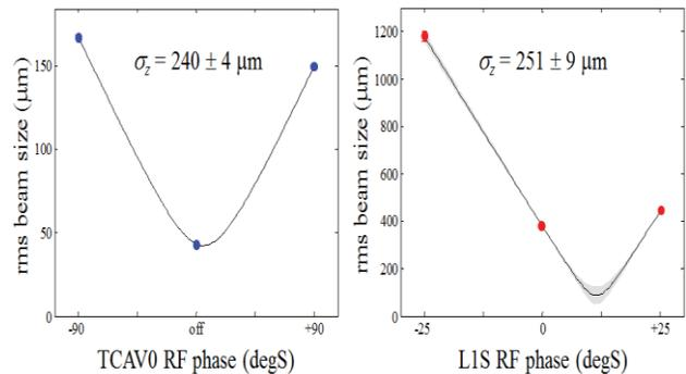
Figure 8: Bunch length measurements in *LCLS* injector exactly as shown in Fig. 7, but now at 40 pC.
