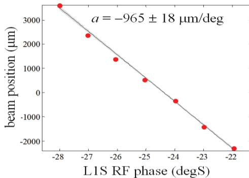
Figure 6: Measured calibration scan where the beam position on the BC1 screen is plotted against the RF phase setting scanned around its  $-25$ -degS nominal phase.
