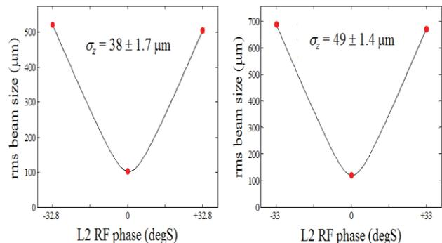
Figure 9: Measured bunch length (RF phasing method in both cases) in *LCLS* just prior to BC2 at 20 pC (left) and 40 pC (right). The transverse RF deflector has not yet been used to confirm this. The rms bunch length values are 38  $\mu\text{m}$  and 49  $\mu\text{m}$ , respectively, and the scale of the beam size data suggests that much smaller values can be measured as well.
