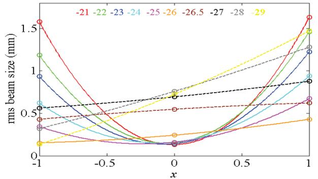
Figure 4: Simulations of bunch length measurements for 10 bunch lengths (color coded w.r.t. Fig. 5 phase). Over-compressed cases (dashed lines) are too linear due to the large chirp,  $h$ , and do not produce precise results.
