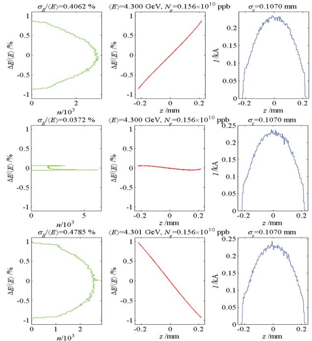
Figure 3: Tracking simulations for  $\varphi = -36.2^\circ$  (top row, nominal),  $\varphi = 0$  (center row), and  $\varphi = +36.2^\circ$  (bottom row), at 4.3 GeV in LCLS BC2 at 0.25 nC ( $\sigma_z = 107 \mu\text{m}$ ). Bunch head is at  $z < 0$  here.
