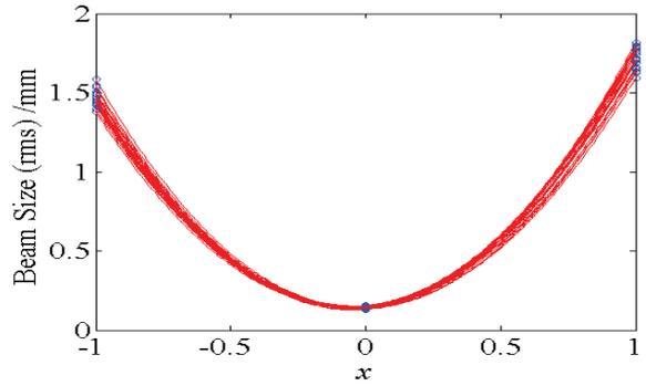
Figure 2: Twenty-five simulated bunch length measurements with parabolic fits ( $\sigma_y$ , not  $\sigma_y^2$  shown) with 5% rms random errors on each beam size measurement resulting in an average rms bunch length of  $106 \pm 3 \mu\text{m}$  (‘true’ value is  $107 \mu\text{m}$ ).
