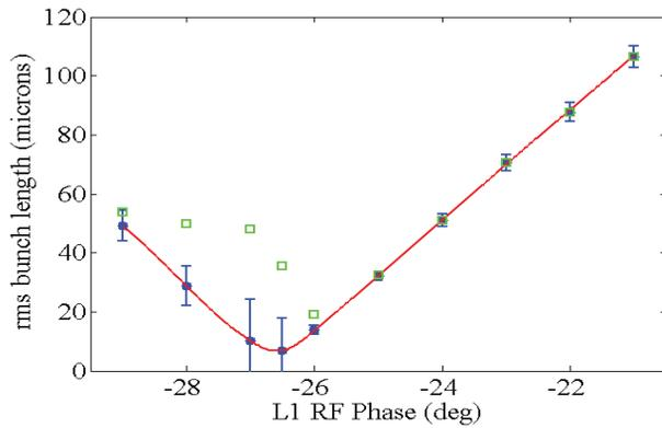
Figure 5: Simulations of Fig. 4 with red curve as tracking results (*i.e.*, ‘true’  $\sigma_z$ ), blue circles as parabolic measurement simulations (which agree well), and green squares as 2-point measurement simulations, which agree only at  $\phi_1 > -26^\circ$ . Error bars, based on 5% rms beam size resolution, show the method diverges for strongly- or over-compressed bunches ( $\phi_1 < -26^\circ$ ).
