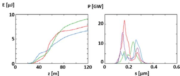
Figure 6: The total energy of the FEL pulse (left) as a function of the distance along the undulator  $z$  for three different shot noises. The power profiles (right) at 60 m for four different shot noises with a clear second spike.
