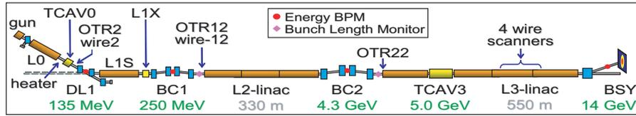
Figure 1: Schematic layout of the LCLS machine.
