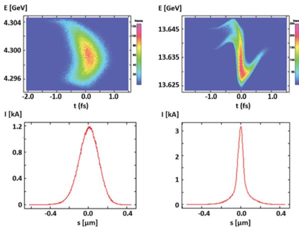
Figure 2: Longitudinal phase space distribution and current profile after BC2 (left) and at the beginning of the undulator (right), for full compression (L2 phase of -32.1°) and a bunch charge of 1 pC.
