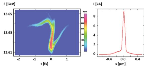
Figure 5: Longitudinal phase space distribution (left) and current profile (right) at the beginning of the undulator for a full compression (L2 phase of  $-32.4^\circ$ ) with a bunch charge of 3 pC.
