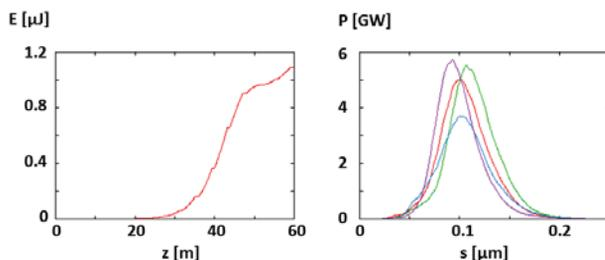
Figure 4: The total energy of the FEL pulse as a function of the distance along the undulator  $z$ , one typical case (left). Power profiles at 50 m for four different shot noises (right).
