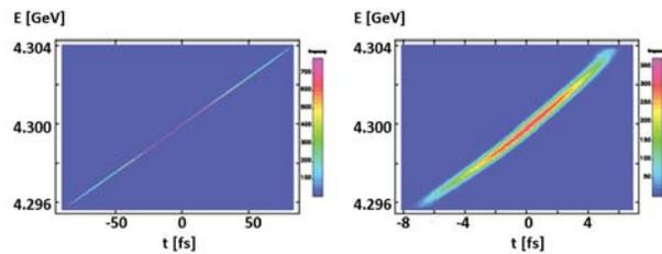
Figure 3: The longitudinal phase space distribution before (left) and after BC2 (right) for under compression (L2 phase of -29.8°) with a bunch charge of 1 pC. The phase space distribution is blown up due to ISR effects.
