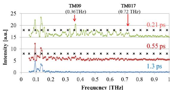
Figure 3: Frequency spectra of CCR for 0.21, 0.55, and 1.3 ps bunch length conditions. Factors and offsets were adjusted for comparison. The theoretical frequencies for  $TM_{0n}$  modes (cross) according to Eq. (1) were shown.
