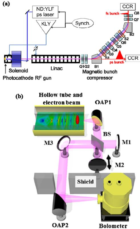
Figure 1: (a) Photocathode RF gun linac with a magnetic bunch compressor of an achromatic arc. CCR is induced by electron bunches from the linac. (b) Diagram of multimode CCR and measurement system. OAP denotes an off-axis parabolic mirror; M, a plane mirror; BS, a beam splitter.
