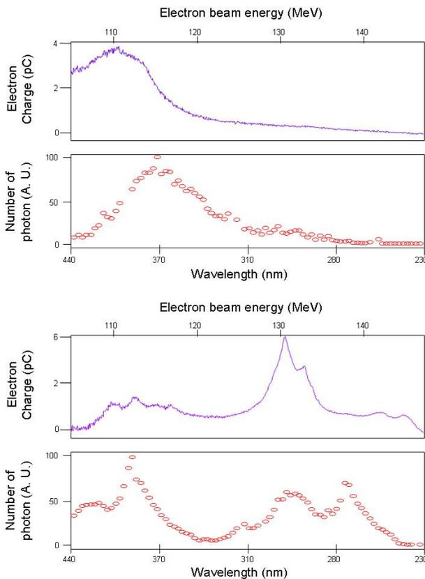
Figure 3: Single shot spectra of photons (red circle) and electrons (violet line) for two different shots.
