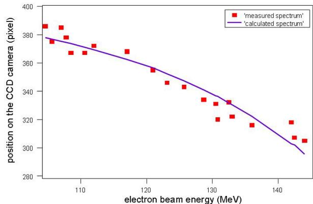
Figure 4: position on the CCD camera of the measured laser light peaks as function of the electron beam energy.
