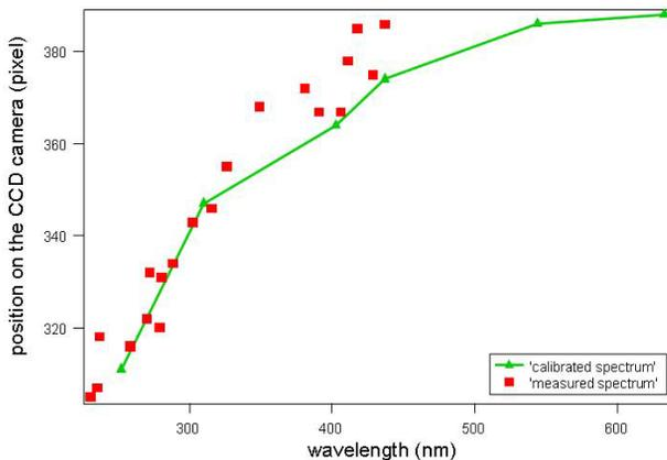
Figure 5: position on the CCD camera of the measured laser light peaks as function of the wavelength.
