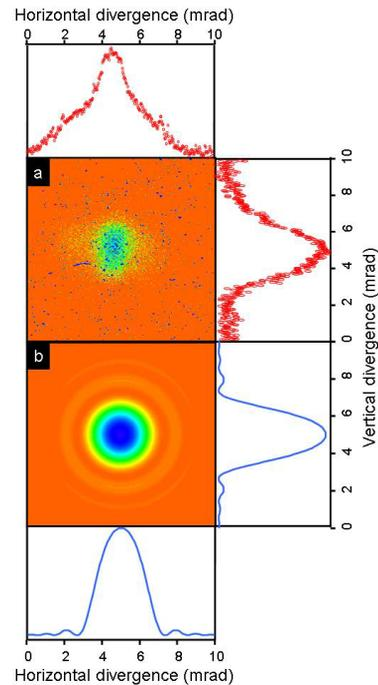
Figure 2: Single shot footprint and corresponding spatial distributions of the radiation measured on the CCD camera. (a) Experimental data. (b) Simulated synchrotron radiation from SRW software [16].
