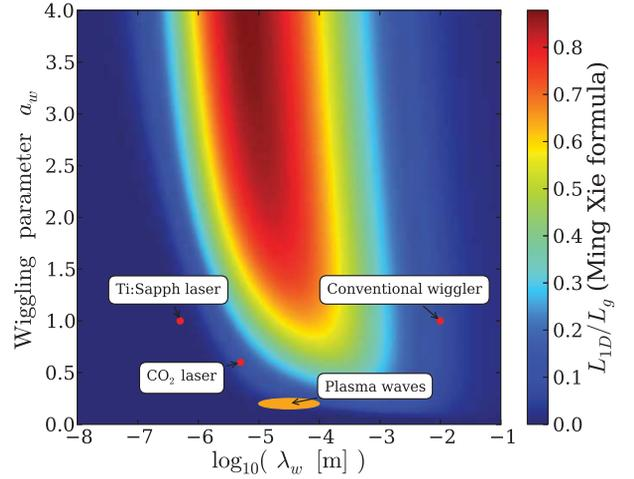
Figure 1: Plot of  $L_{1D}/L_g$  (as given by the Ming Xie formula) as a function of the wiggling parameter  $a_w$  and the wiggler period  $\lambda_w$ .
