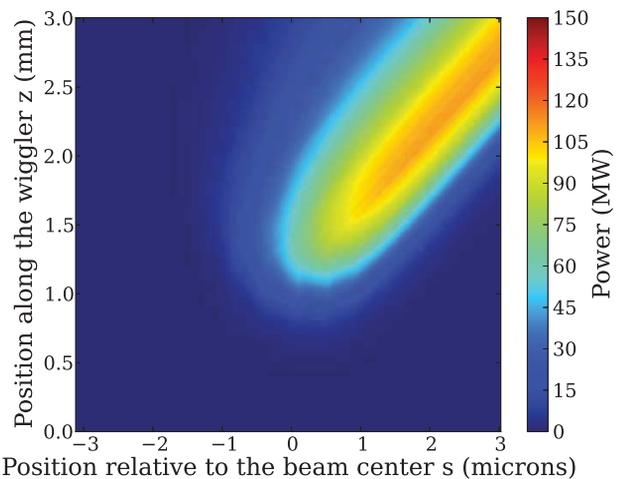
Figure 3: Radiation power along the wiggler in the case of a freely expanding electron bunch
