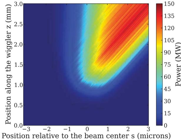
Figure 4: Radiation power along the wiggler in the case of a periodically refocused electron bunch
