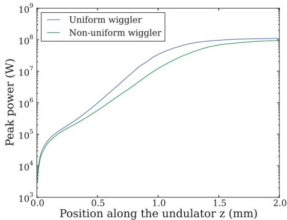
Figure 5: Evolution of the peak power of the FEL radiation along the wiggler for a uniform wiggler and non-uniform wiggler obeying equation (8) with  $Z_R = 2$  mm.
