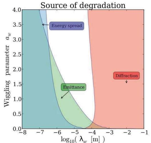
Figure 2: Range of parameters (in terms of wiggling parameter  $a_w$  and wiggler period  $\lambda_w$ ) in which each source of degradation becomes important.
